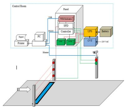
Weigh Inmotion Software (WIMSoft) is dynamic weighing software for weighbridge vehicle weight management in the field of Mining, Logistics, Industrial Plants, Ports, Toll gates and Roadways Industries as private and public usage. It can be used for all type of vehicle **weighbridges**, **axle** weighbridges and wheel **weighing pads**. It can transfer data to Cloud, Shared or Main server database in online and offline mode.
